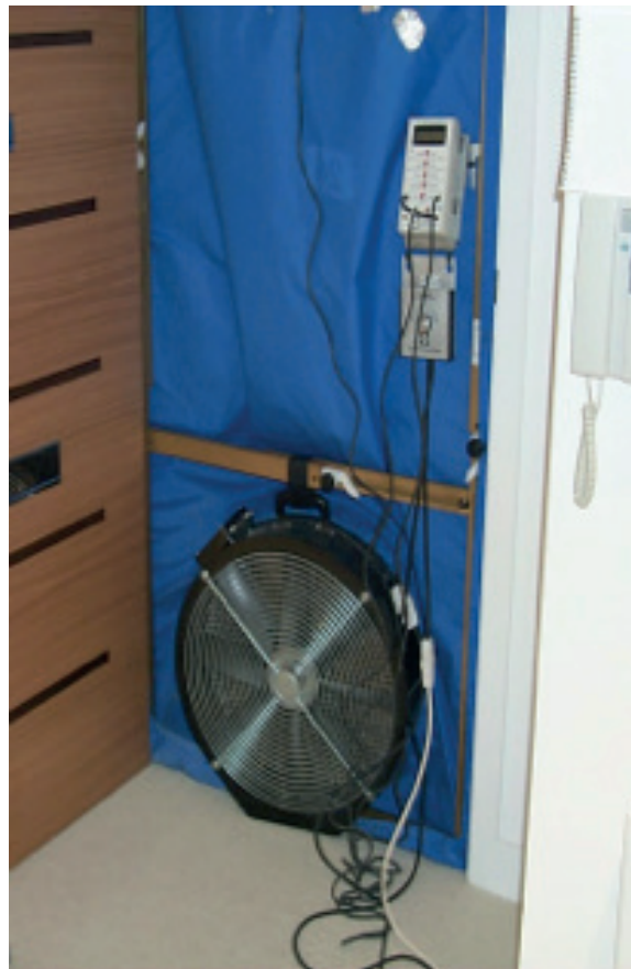
Figure 11 Air pressure testing fan installed in the entrance doorway of a building
