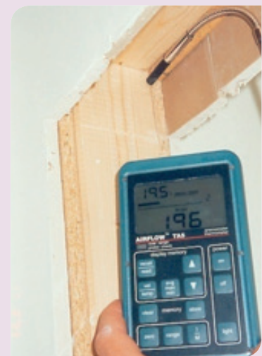
Figure 17 Thermo-anemometer used to detect air leakage paths
